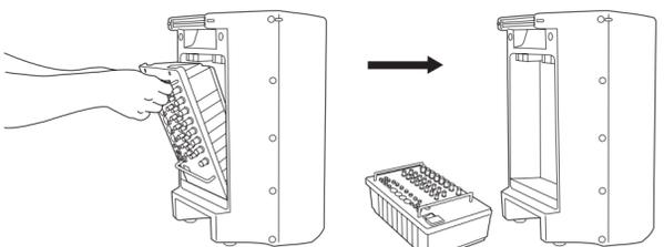
**Caution** Use only the mixer's handles when removing the mixer from the speaker and when carrying the mixer separate from the speaker.
