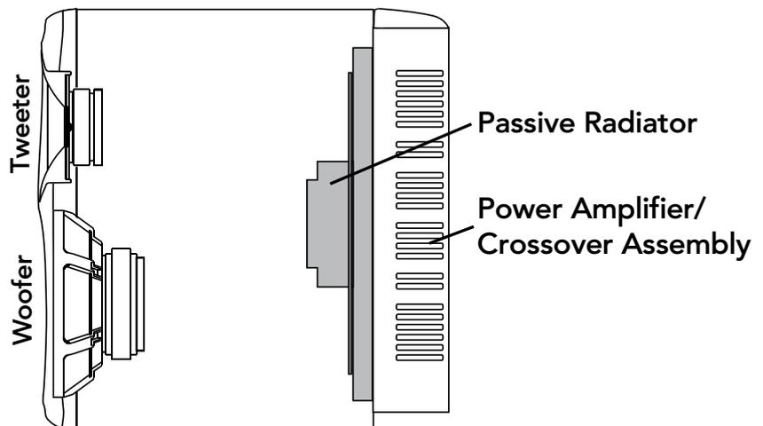
Figure 1. HR624 MK2 Cutaway side view
